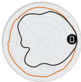
Figure 3. 5GHz Azimuth Antenna Patterns
