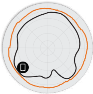
Figure 2. 2.4GHz Azimuth Antenna Patterns
